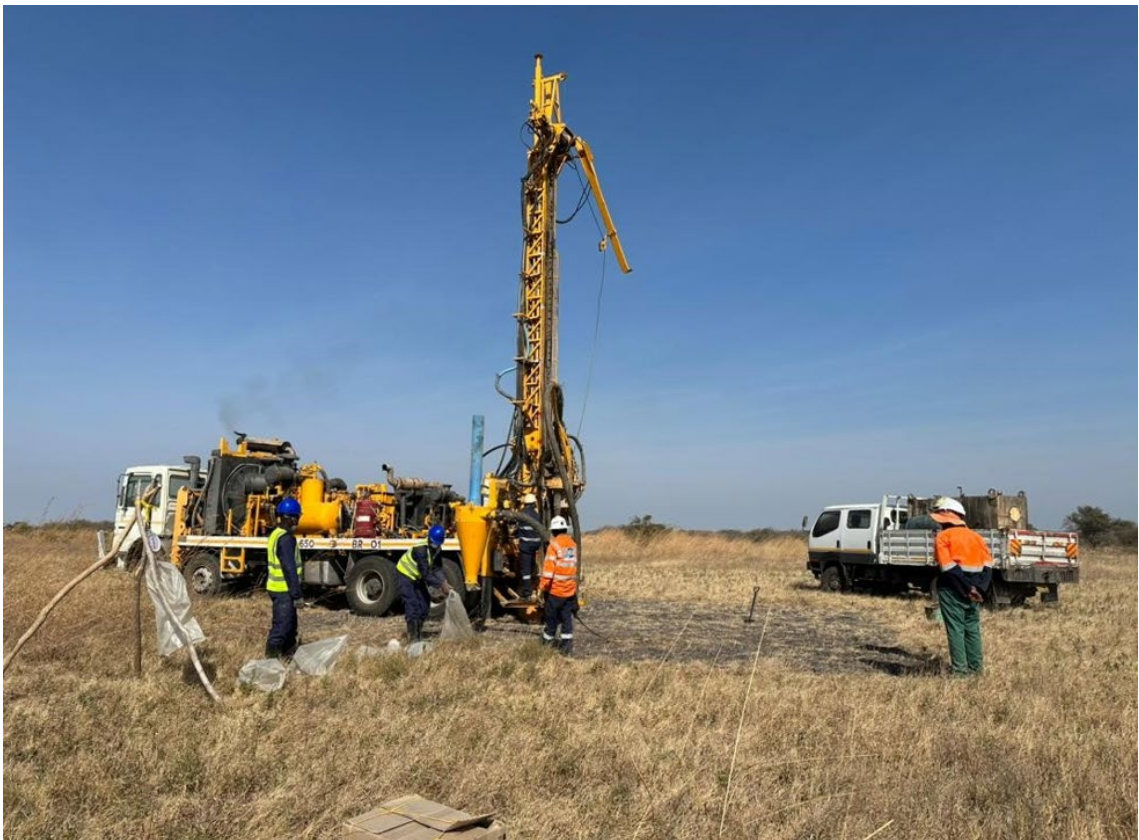
Figure 3 – Air core drilling rig at Itigi
