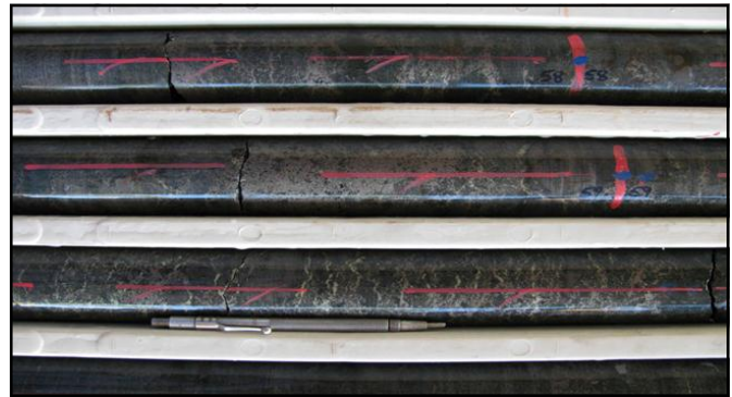
Photo 1. MKED004, ~57.00 to 60.00 metres - Strong fracture controlled pyrrhotite + pyrite + chalcopyrite mineralisation in a garnetite and diopside calc-silicate units. Assays returned for interval: 3m @ 1.04% copper, 361ppm cobalt and 0.09g/t gold.
