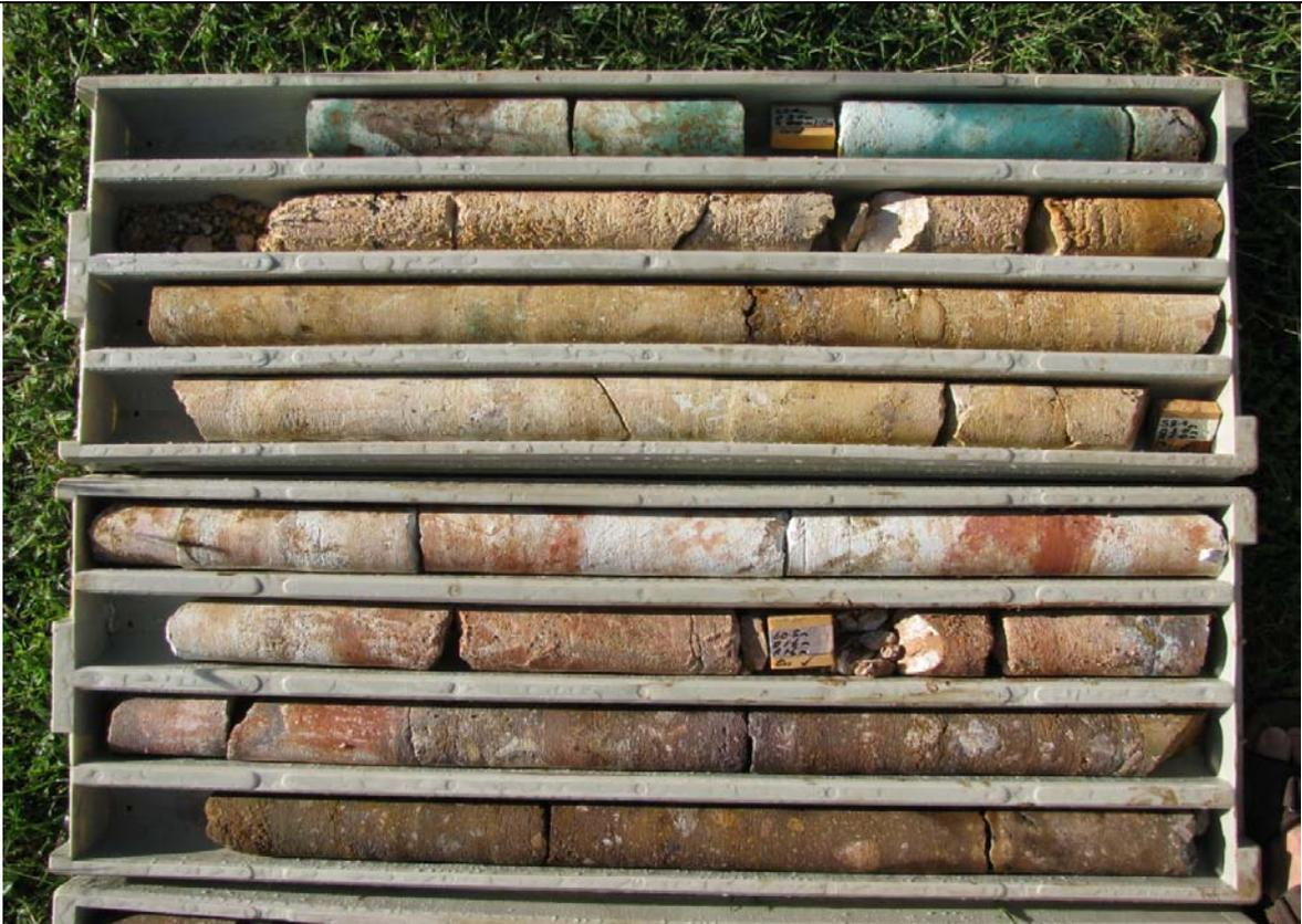
**Figure 1.** MDD006 – Core recovered in the target breccia from 55.5 metres and continues at depth beyond 62 metres as shown. Yellow brown rock in bottom metres is supergene Chalcocite (Copper Sulphide) breccia from 60.5 metres confirms the extension at depth of the Mt Dorothy sulphide breccia.
