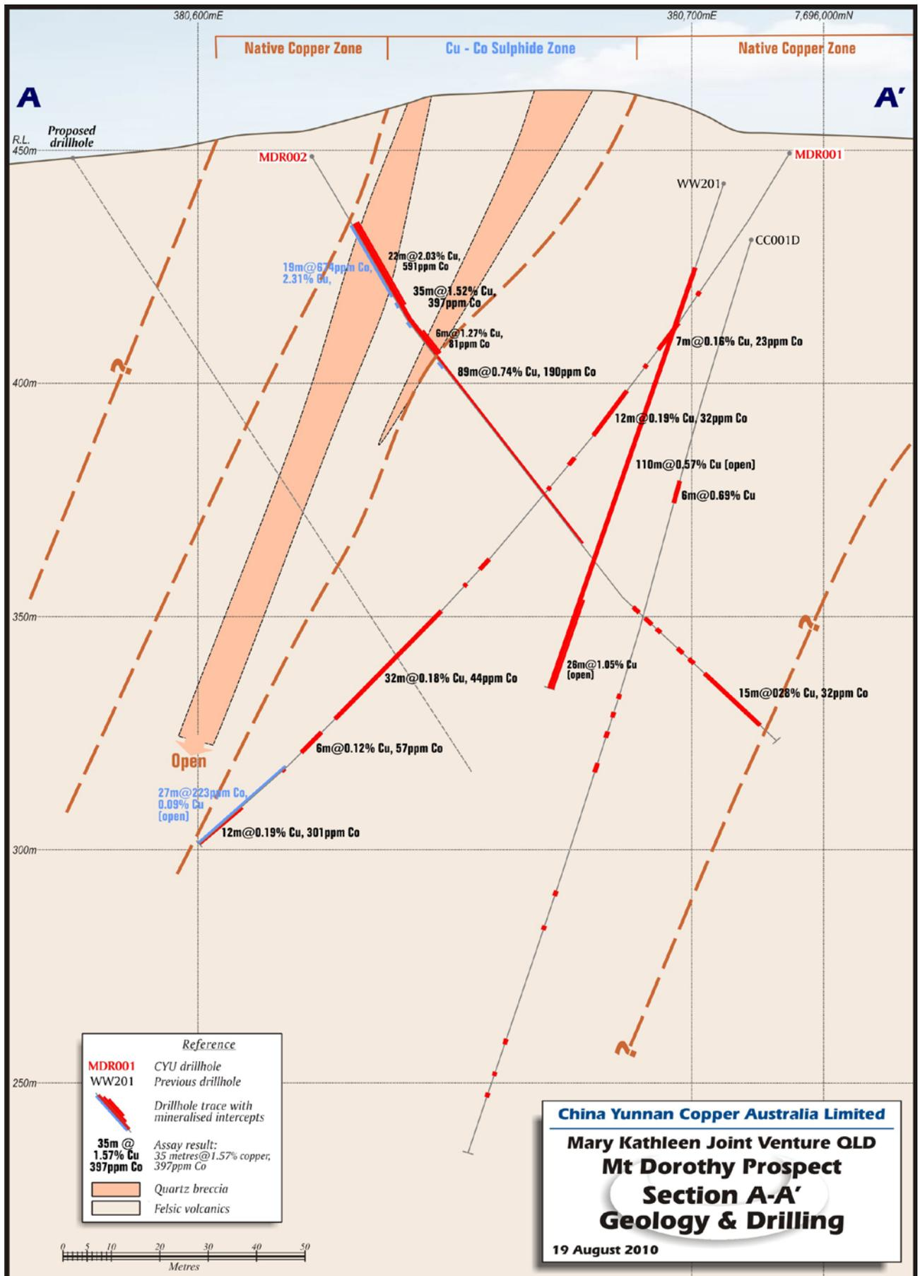
Figure 3: Mary Kathleen JV: EPM 14019 – Section A-A' looking north-northeast highlighting the broad copper mineralisation intersected in MDR001 and MDR002.
