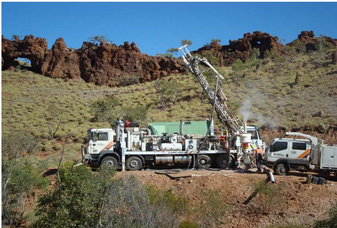
**Plate 1:** Mary Kathleen JV: EPM 14019 –RC Drill Rig drilling MRD001, looking south. Outcrop in the background is the surface expression of gossanous quartz breccia outcrop extending for >500m strike length.
