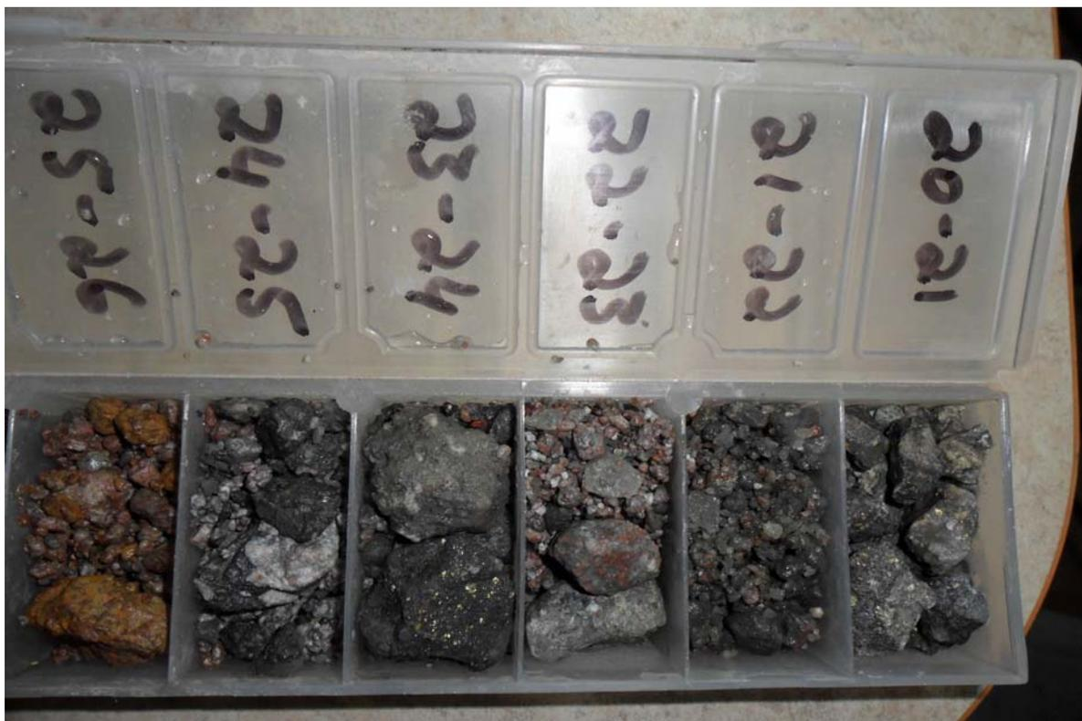
**Plate 2:** Mary Kathleen JV: EPM 14019 – MDR002 shallow visible primary sulphide mineralisation in RC drill chips. The interval 20m – 25m returned assays of 5m @ 3.15% copper, 1,473ppm cobalt.
