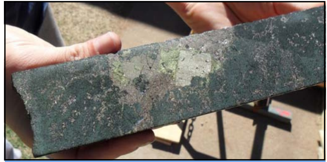
Photo 1: MKED008 ~504-505 metres: Disseminated pyrrhite + chalcopyrite + pyrite mineralisation in garnetite and diopside calc-silicate.
