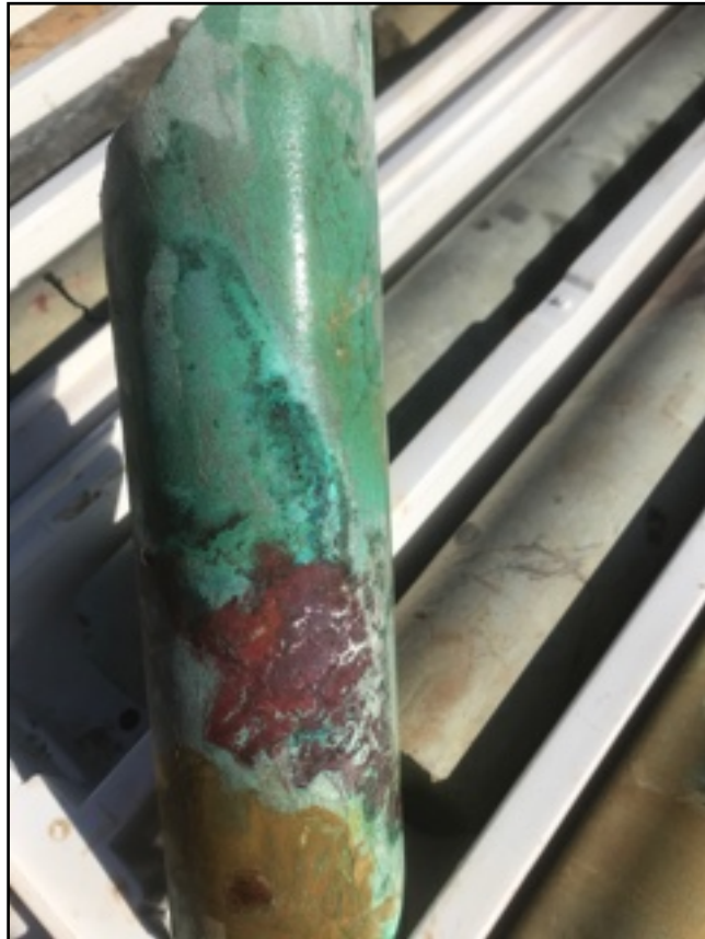
Figure 4 – Diamond core sample from current drill hole AORD004 at Onedin (assay results are pending) showing rich copper oxide mineralisation – malachite and cuprite
