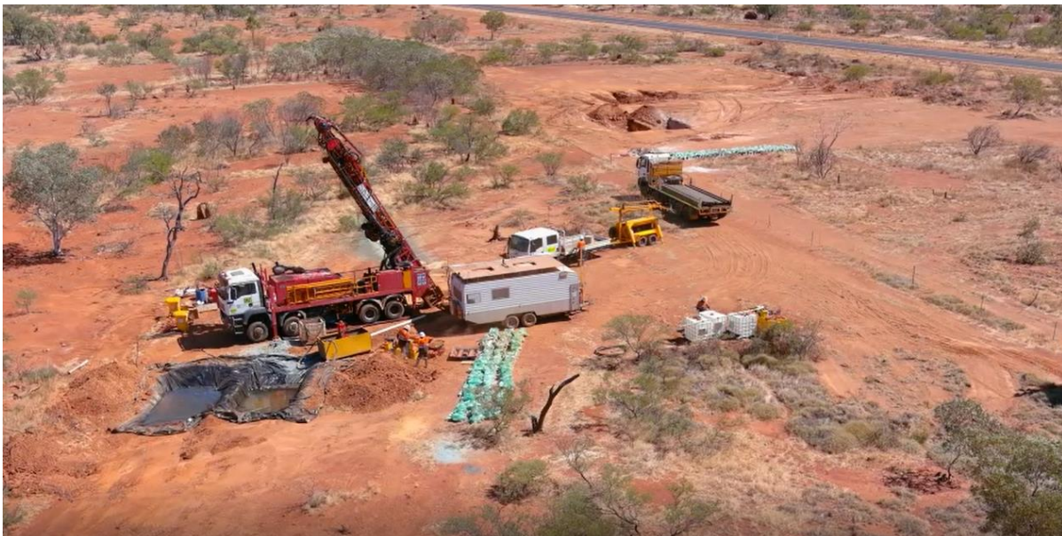
Figure 1 – Diamond drilling at Sandiego
