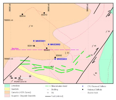
Figure 2. Drillhole Location Plan.
