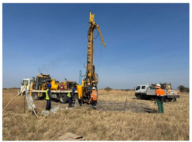
Figure 3 – Air core drilling rig at Itigi
