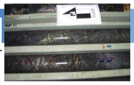
MKED036 – ~188m - Elaine copper-gold resource – patchy disseminated sulphide mineralisation dominated pyrrhotite + chalcopyrite +/- pyrite
